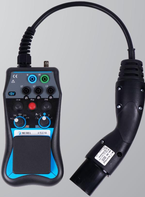
The A 1532 EVSE XA adapter is used for verification of electrical safety and functional testing of EVSE together with supported METREL installation testers. It is intended for testing Mode 3 EV supply equipment with a type 2 connector. XA version supports 3 phase load testing up to 13 A and different error types, including PE open.
