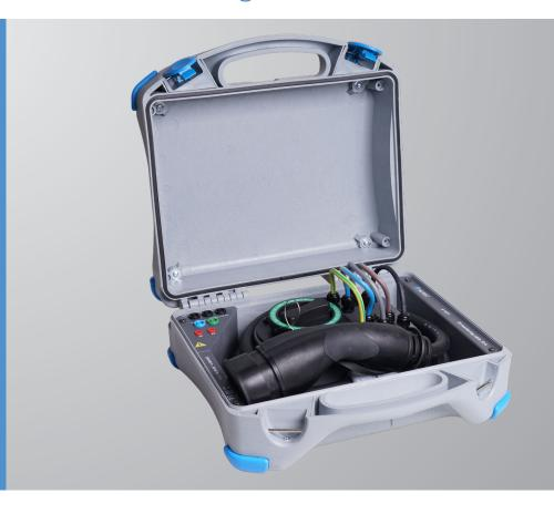
The A 1631 EV monitoring cable is a special accessory designed for CP signal, current and voltage monitoring during Electric Vehicle (EV) charging process in conjunction with supported Metrel testers and adapters. It is equipped with a Type 2 female plug connector to connect to an EV and a Type 2 male socket outlet for connecting to Electrical Vehicle Supply Equipment (EVSE).
